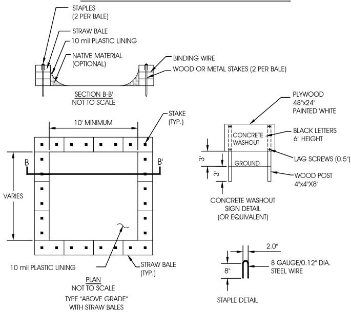
CONCRETE WASHOUT NOTE: CONCRETE WASHOUT OPERATIONS SHALL TAKE PLACE WITHIN THE PROPOSED PROJECT AREA UTILIZING THE CONTRACTOR'S PORTABLE CONCRETE WASHOUT CONTAINER OR WITHIN A BERMED/CONTAINED AREA. CONTRACTOR SHALL TAKE ALL NECESSARY MEASURES TO ENSURE WASHOUT MATERIAL DOES NOT LEAVE THE WASHOUT AREA OR ENTER THE STORM SYSTEM. CONTRACTOR SHALL CLEAN UP AND PROPERLY DISPOSE OF ALL LEFTOVER WASHOUT MATERIAL.
