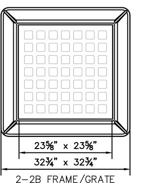
2-2B FRAME/GRATE NEENAH R-3405-W (TYPE H GRATE) EJIW NO. 5250 (TYPE M GRATE)
