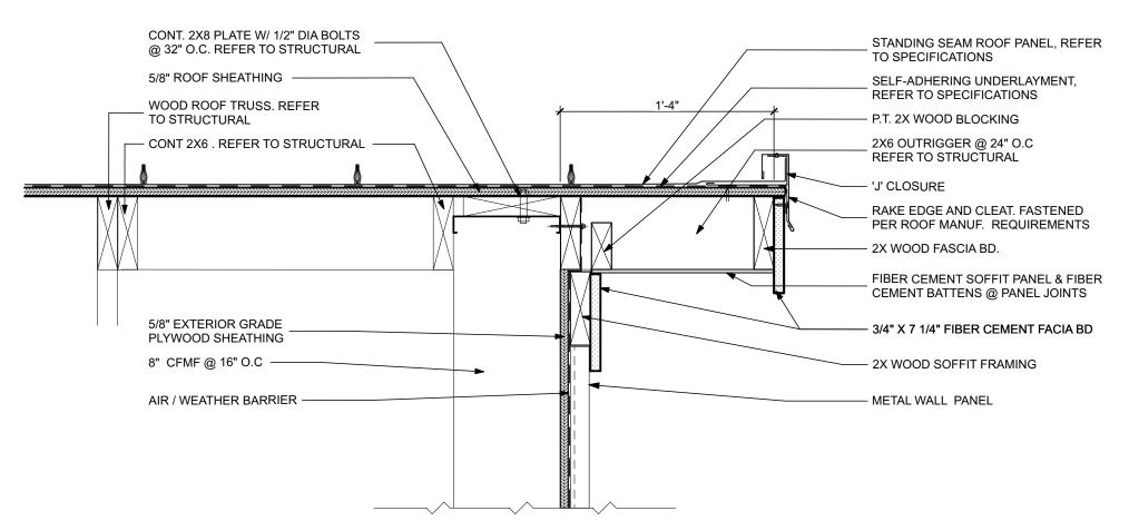
RAKE DETAIL SCALE: 1 1/2"= 1'-0"
