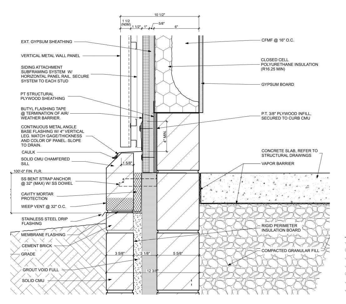
TYPICAL WALL BASE DETAIL - GARAGE SCALE: 3" = 1'-0"
