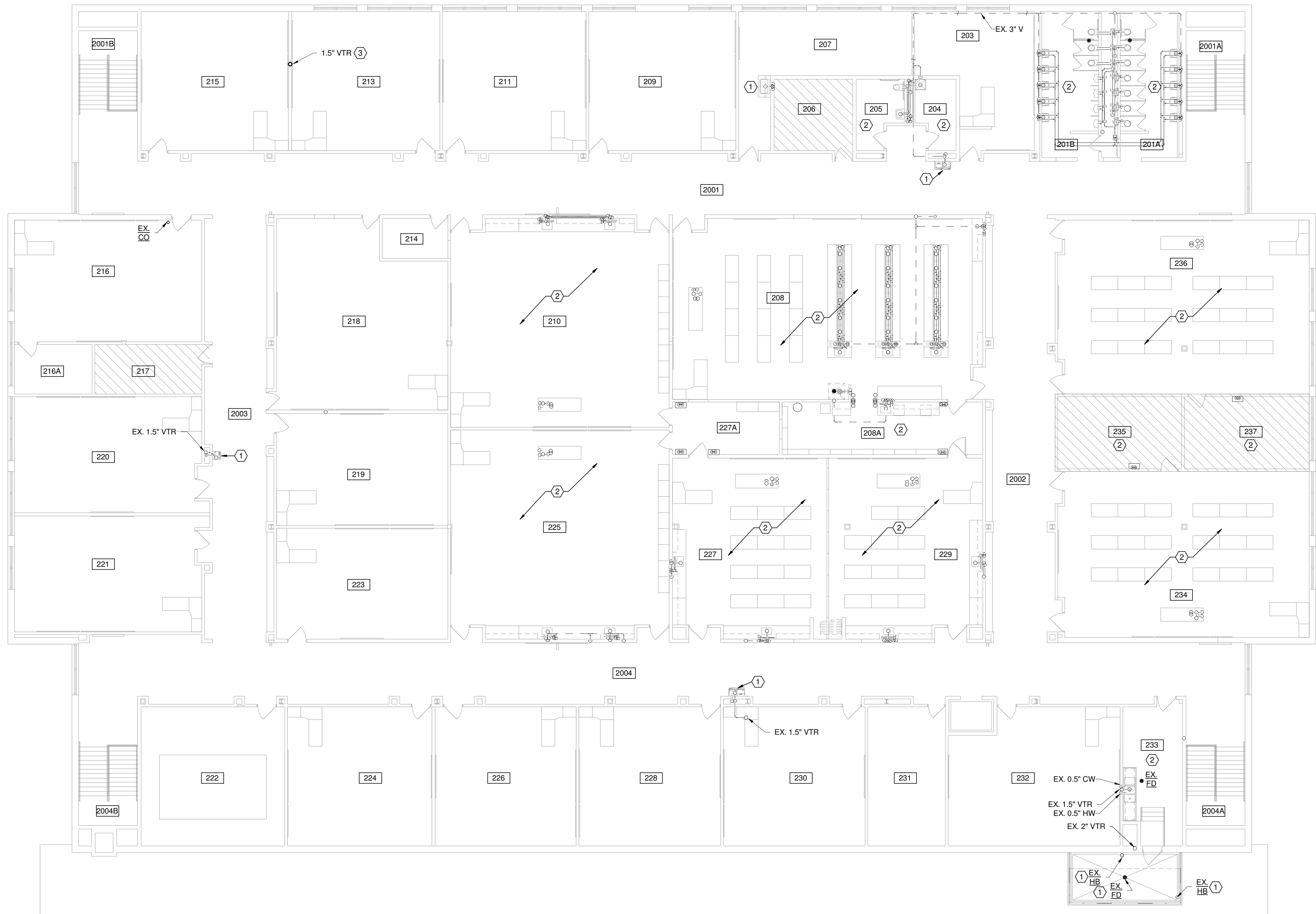
1 SECOND FLOOR OVERALL PLAN - DEMOLITION 3/32" = 1'-0"
