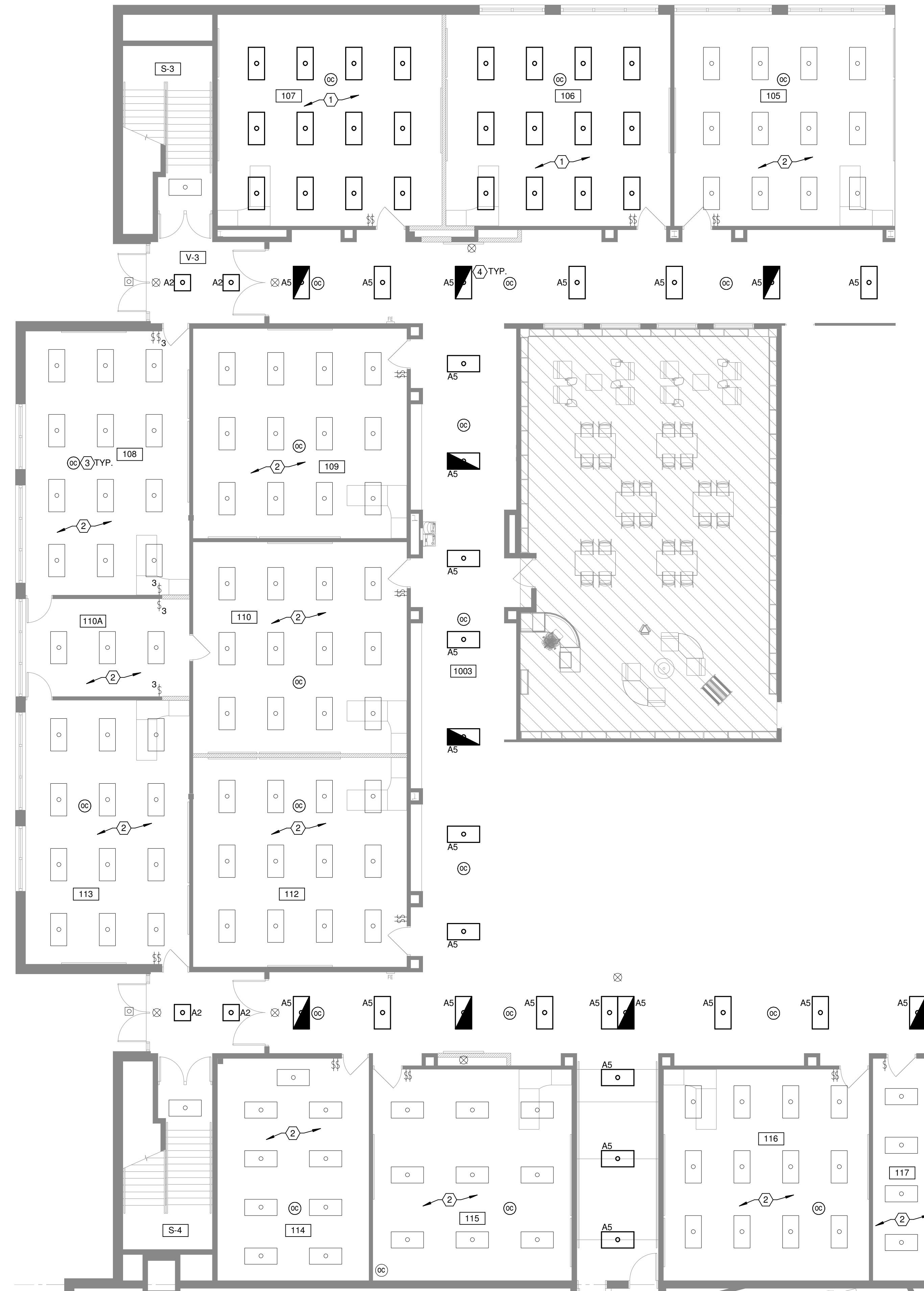
1 FIRST FLOOR LIGHTING PLAN - NEW WORK - SOUTH 1/8" = 1'-0"
