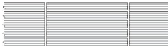
Reveals (1") can be **Symmetrical** giving a linear appearance or **Staggered** to minimize joint layout
